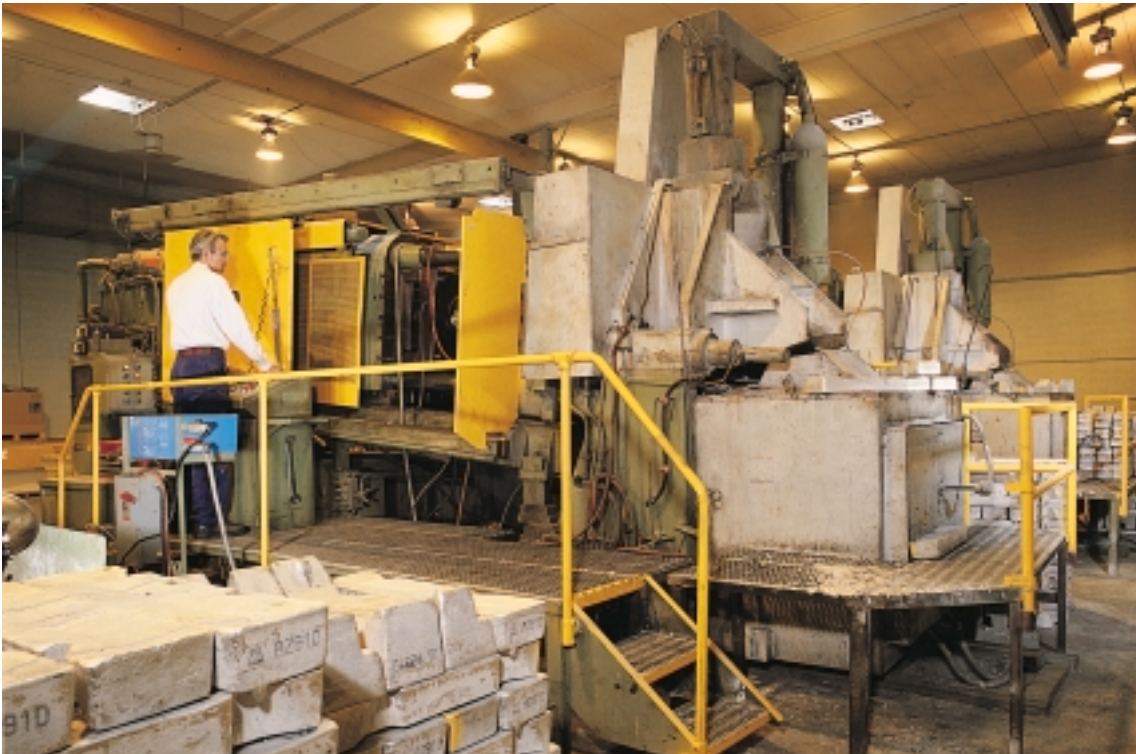
Three of among the world's largest hot-chamber Mg die casting machines, 650-ton Frechs (left), cast 24 in. x 24 in. (60.9 x 60.9 cm) Mg parts using the more cost-efficient hot-chamber process.
