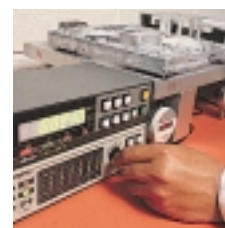
This electronic flatness tester is used to verify a critical flatness tolerance to \pm .0005 in. ( \pm .0127 mm).
